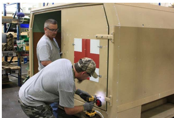
Rock Island Arsenal-Joint Manufacturing and Technology Center (RIA-JMTC) employees install the rear doors of an M997A3 Ambulance.
