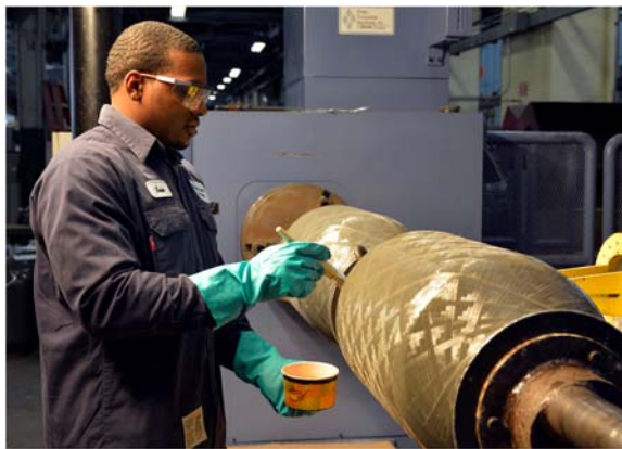
Watervliet Arsenal metal processor applying a gelcoat to a lightweight bore evacuator for the Abrams tank system.
